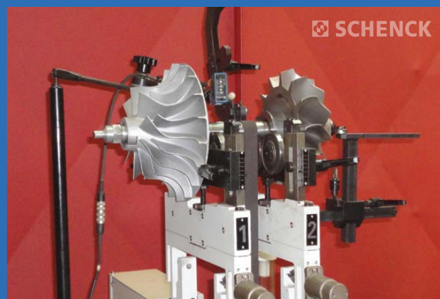
Schenk HBU 20/40 Balancing Machine, quality grade G2.5 (DIN-ISO 1940-1)
